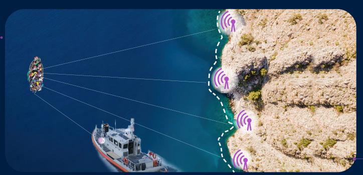
The proposed solution simulates a cellular network signal, effectively attracting cellular devices in maritime areas. Subsequently, the received signals are analyzed to ascertain the distance between the cellular device and the system. This analysis enables the determination of a range to the detected cellular device. As a result of the collaboration between various units within the system, the source of the signal can be triangulated.
