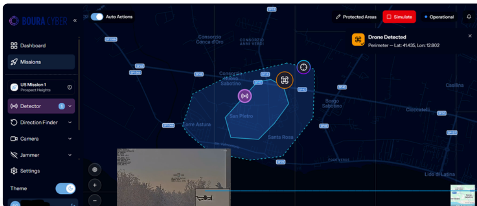
Manual camera cueing from the C2 system to obtain visual confirmation of an unauthorized drone.
